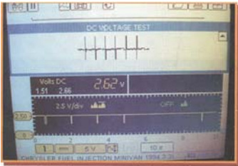
Photo 5: The voltage graphing displayed on the Vantage Pro is a real-time electrical signal. In contrast, the voltage graphs from the SOLUS indicate trends in the serial data stream.
